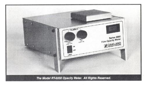
Ideal for the laboratory or plant floor, the model RT-6000 is a simple-to-use, off-line instrument that indicates relative opacity of plastic film, paper, laminates, printed packaging and other materials. With a single pass of the light source through your material, the system measures relative light transmission on a scale of 0 to 100 Opacity Units, representing perfectly transparent to purely opaque materials, respectively.
